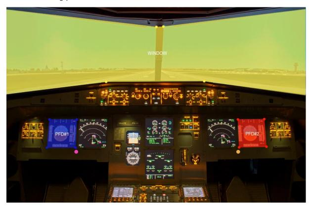
Improvement of training quality in flight training industry is a continuous demand for the participants. Flight simulation is an inevitable component of practical flight training, the development of its subsystems can add new features that serves the essential goal. Project NGFNPT develops an eye tracking based platform for multi-crew flight decks to support regular Multi Crew Cooperation trainings with advanced technology, providing objective measurement data for flight instructors.
